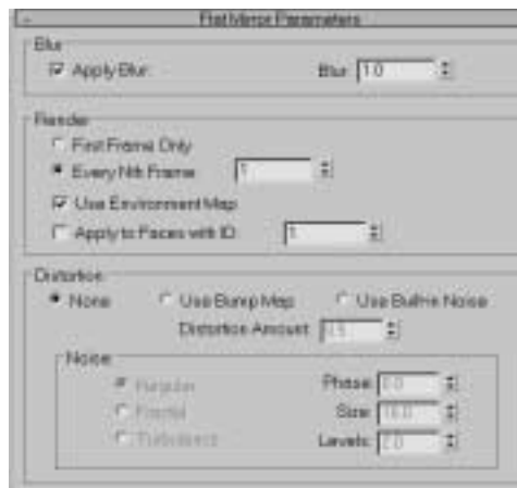
Figure 14.65 The rollout for a Flat Mirror map allows you to add an Environment map to the reflection, and to disturb the reflection with noise or a Bump map.
