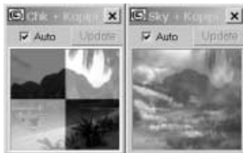
Figure 14.25 Mixing a Bitmap with a Checker map (left) and another Bitmap (right).
