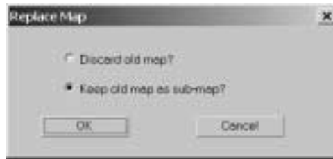
Figure 14.27 Choosing to keep a map as a sub-map adds another level to the material tree.
