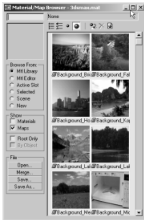
Figure 14.3 As you choose each Browse From option, the maps that are available at that location appear in the Material/Map Browser.
