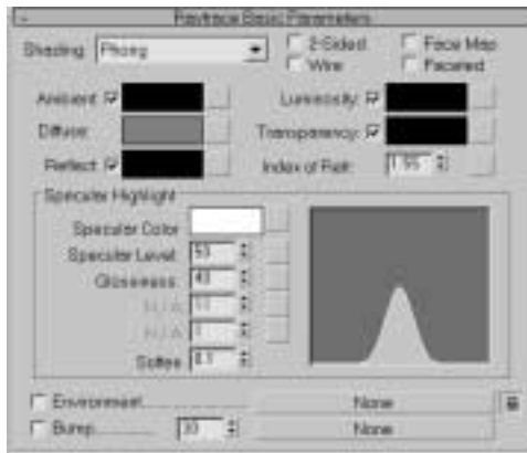
Figure 14.74 Setting Transparency to white is the same as making an object 100% transparent.
